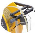
To avoid damaging the tape on the side of the casing, hang the dipper-See EXAMINER on the casing (1) and run the tape over the guide on the frame leg (2). If you cannot hang the unit, drape a soft cloth over the edge of the casing, guide the tape down the center of the well away from the side.
