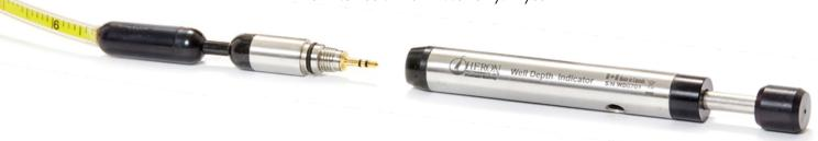
The Well Depth Indicator Probe (or bottom detector) is used to measure full depth in wells and boreholes. The Well Depth Indicator Probe uses a pressure sensitive plunger to measure the distance to the bottom of the well. When the Well Depth Indicator Probe reaches the bottom of the well, the plunger enters the probe body closing a switch, initiating an audible and visual signal at the top of the well. The well depth reading is taken directly from the tape.
