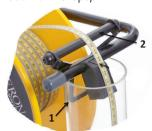
• To avoid damaging the tape on the side of the casing, hang the dipper-See EXAMINER on the casing (1) and run the tape over the guide on the frame leg (2). If you cannot hang the unit, drape a soft cloth over the edge of the casing, guide the tape down the center of the well away from the side.
